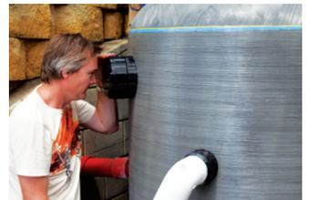
*Generally, large manholes and sight glasses are harder to incorporate in high pressure filters, because any opening in a filter vessel creates a potential weak point or complicates the manufacturing process.*
